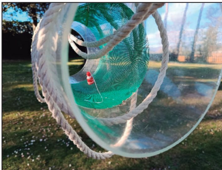
Figure 6. Methacrylate cylinder wrapped with rope, with a pheromone septum suspended inside.
